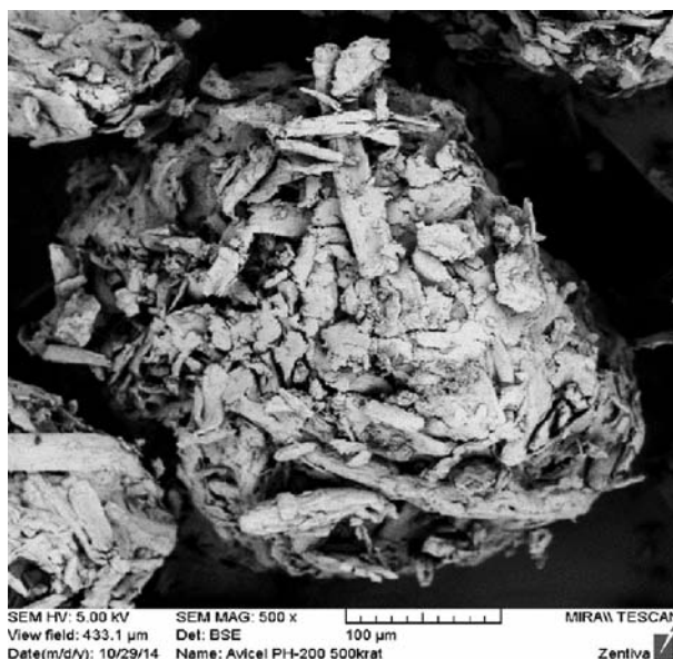
Fig. 1. SEM image of Avicel PH-200 particle, magnification 500x
